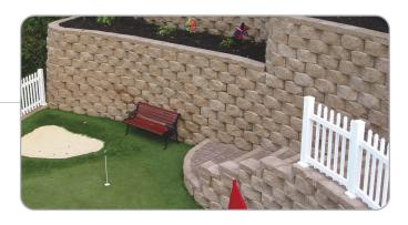
structure is constructed from Keystone Compac straight-faced treads, capped by Keystone Universal capping units. For a nice finishing touch, with the safety of his grandchildren in mind, Waletich added white fences to the top of the pedestrian-accessible walls. The fences are attached to the Keystone Universal capping units with masonry anchor screws and construction adhesive.
